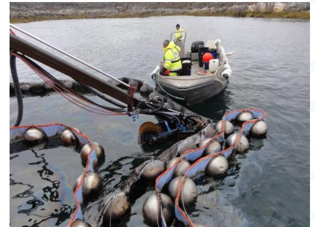
Shoreline experimental in situ burning experiment in GRACE project. Source: Aarhus University
