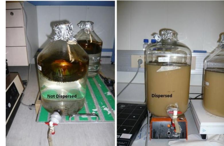
Nondispersed and dispersed oil in laboratory scale experiment.
